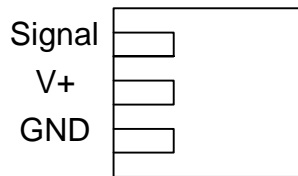
Gambar 2 Pin Out Kabel Motor Servo
